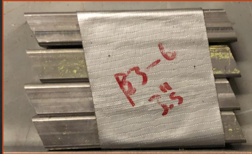
Figure 12: Finished Cut \frac{1}{2} " Sq. Tube Pieces at an Angle [2]
