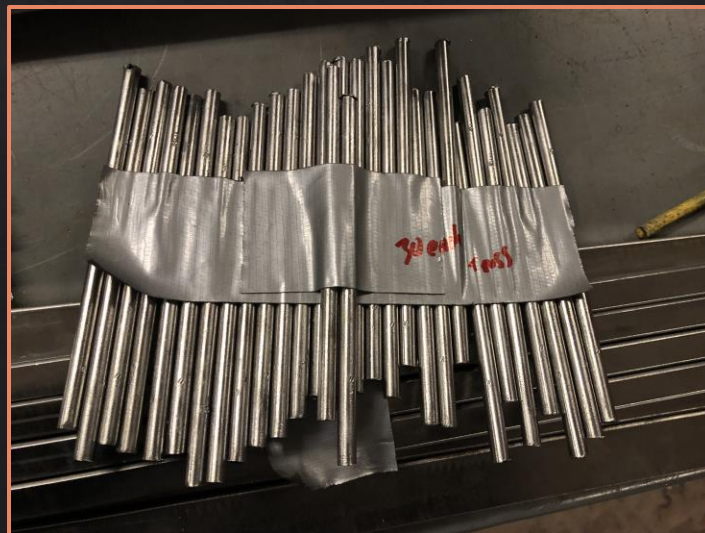
Figure 13: Finished Cut & Cleaned \frac{3}{16} " Rods [2]
