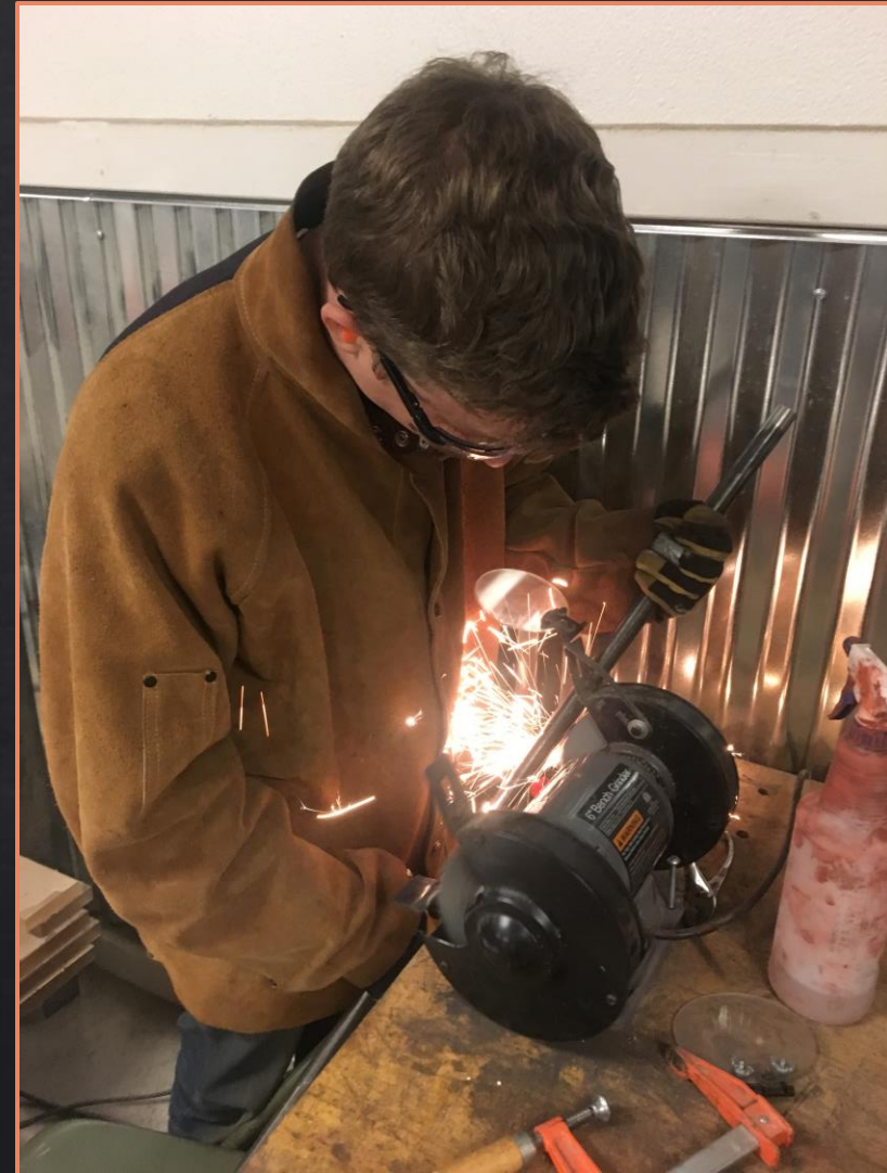
Figure 14: Andrew Preparing Steel Member for Welding [2]
