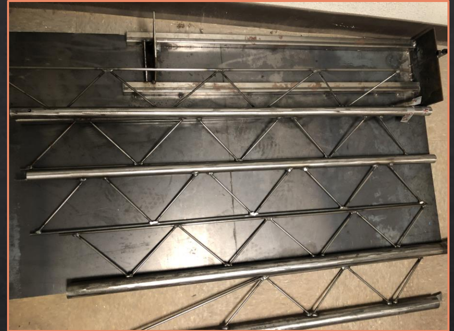
Figure 17: Welded Superstructure Members [2]
