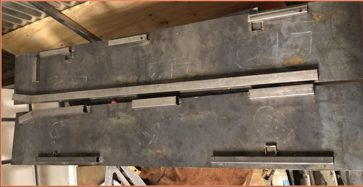
Figure 15: Jigs for Superstructure Members [2]
